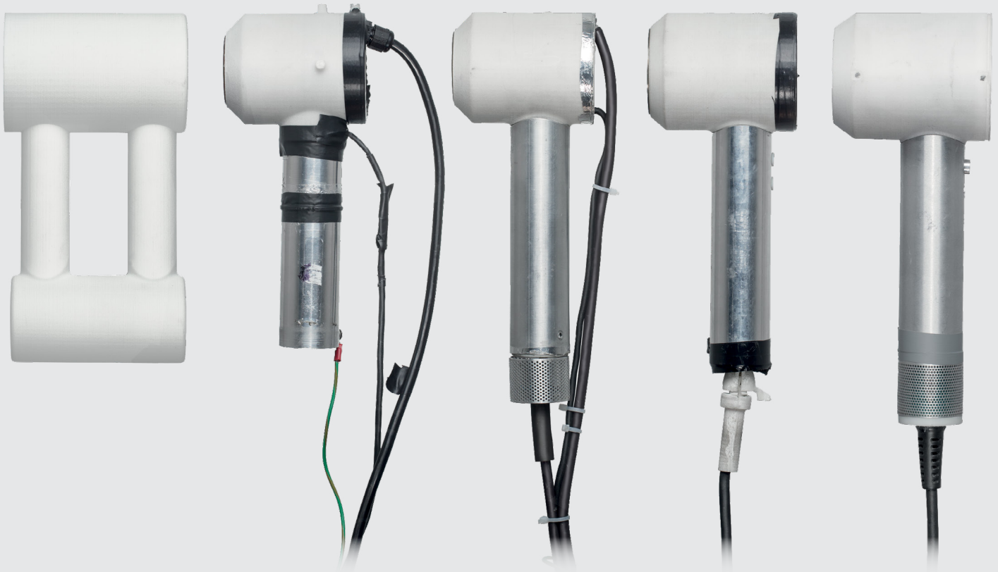
B - rig 1st fully integrated rig with V9 motor, heater and electronics
